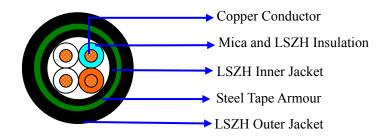
**Conductor:** Plain Annealed Solid Copper to IEC 228 Class 1
